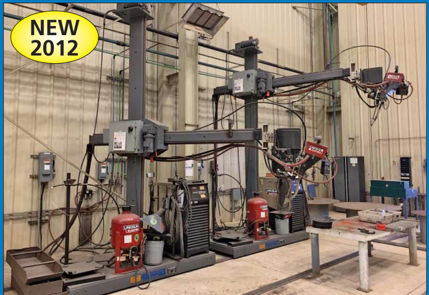
(4) 9' x 9' Preston-Eastin Model MA99AMD Welding Manipulators w/ 1,000-Amp Lincoln Power Supplies
