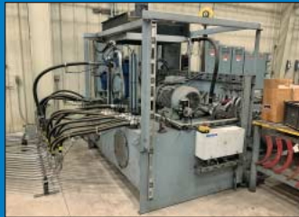
3.54" x 120" Haesler Model VRM-hy 3050-997 Four-Roll Hydraulic Plate Roll
