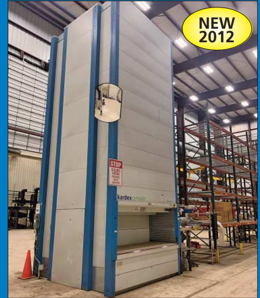
Kardex Remstar Model Shuttle XP-500-2450x864US Automated Storage and Retrieval System
