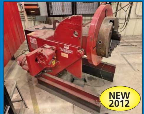
(6) 3,000 Lb. Pandjiris Model 30-6 FB Motorized Tilting and Rotating Weld Positioners
