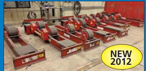
(5) 30/45 Ton Weldwire Model WWRI-30 Tank Turning Roll Sets
