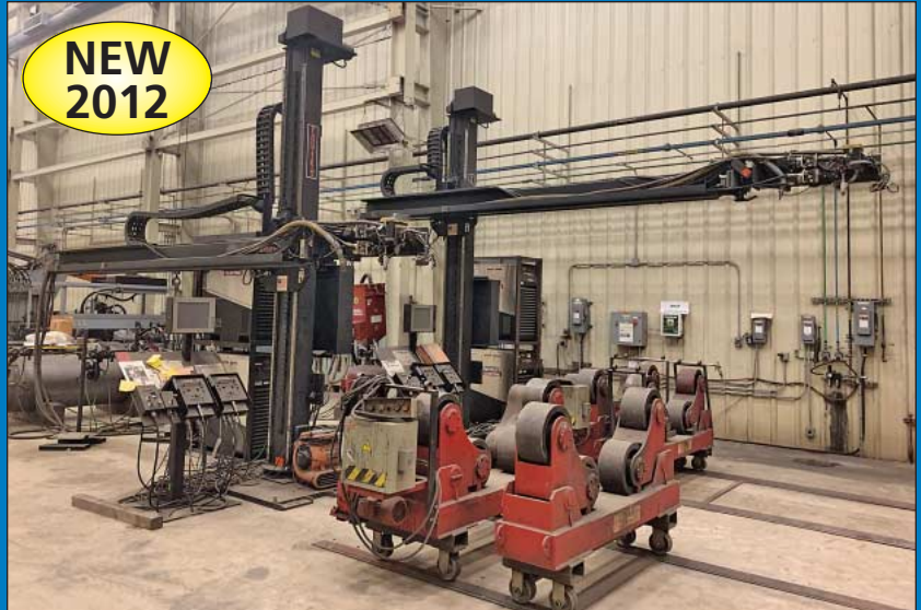
(2) 11' x 11' Pandjiris Model 1100 Welding Manipulators w/ Dual 1,000-Amp Lincoln Power Supplies
