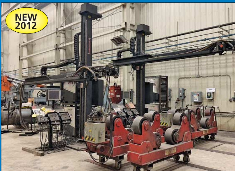
(2) 11' x 11' Pandjiris Model 1100 Welding Manipulators w/ Dual 1,000-Amp Lincoln Power Supplies
