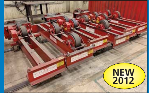
(16) 45 Ton to 10 Ton Weldwire Tank Turning Roll Sets
